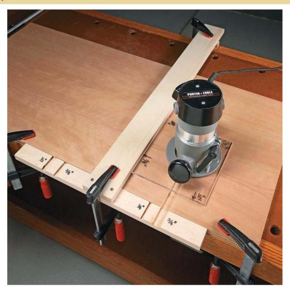
Routing dadoes and grooves with a shopmade T-square works great. The setup is quick and easy. But most T-squares are usually made for a specific diameter of router bit. The auxiliary router base and T-square you see here solves that problem. This allows me to accurately position and rout four sizes of dadoes and grooves by simply rotating the router.
