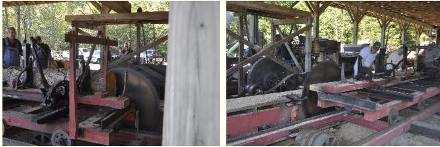
Left - Log Encountering The Saw Blade    Right - Log Exiting The Saw Blade
