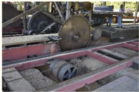
Left - Sawyer In Foreground, Hydraulic Men In Back    Right - Pulley & Blade, Pulls The Log Into The Blade
