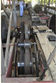
Left - Power Plant Right - Pulley And Belt System For Sled, Blade & Saw Dust Removal
