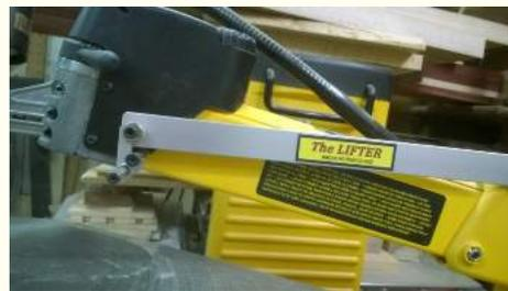
I have one installation recommendation to keep your scroll saw looking great. Use a rotary tool with a sanding drum to expose the bolt head under the plastic switch cover. This allows the installation of the latch anchor. See caption in the photo. It makes for a professional look as if "The Lifter" came with the DW 788. Happy scrolling!
