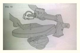
Now, this unique device holds the DW 788 scroll saw upper arm in the full up position eliminating the need for the scrap block. This frees-up both hands to thread the blade through the hole. Then it is a simple matter of lifting the upper arm and releasing the latch assembly and reinstalling the blade into the upper blade clamp of the scroll saw. It is easy, fast, simple, and reliable! All for \$30!!
