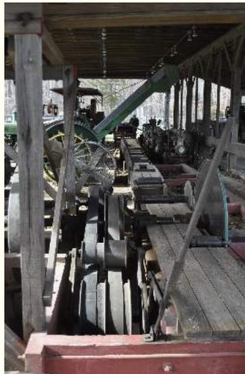
**This View Shows The Belt Drive System For The Saw Blade**
