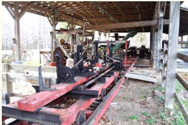
**A Look Down The Rail Road Style Conveyor That Brings The Logs Past The Saw Blade**
