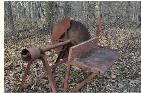
**Belt Driven Chop Saw? Pushing The Handle Forward Raises The Board Into The Blade To Cross Cut The Board**
