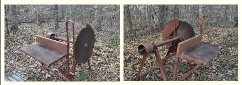
Belt Driven Chop Saw? Pushing The Handle Forward Raises The Board Into The Blade To Cross Cut The Board
