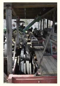
This View Shows The Belt Drive System For The Saw Blade
