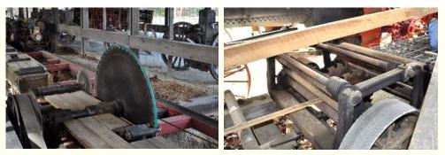
Photo On The Left: Detailed View Of The Saw Blade. Note The Splitter Behind The Blade.
