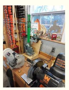
• Hand powered grinder - It's amazing how this simple piece of equipment can quickly remove metal, and yet minimize the potential for burning the tool. Note that the grinder and metal vise are mounted on boards so that they can be clamped where desired; even on a pickup truck tailgate!
