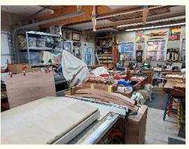
• The cabinet maker's bench (from Wooster, Ohio) with tail and face vises is the primary workstation. The large center drawer contains the small tools most frequently used (i.e. rules, small saws, chisels, wood files). Note that behind the bench is a spindle sander and stool with fan. The spindle sander is infrequently used, so putting a little stool over it makes a nice platform for the fan. Essentially, an efficient use of space.
