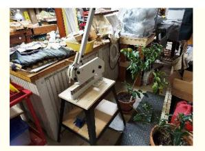
• Plate shear - great for modifying hardware and cutting plate (i.e. old handsaw blades) to create scrapers.
