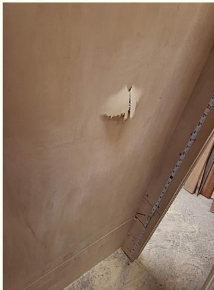
**View Of Backside Of Plywood Where The Maple Kickback Penetrated The Plywood Sheet**
