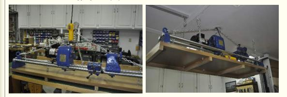
Views Of Record Power Lathe On Work Bench (Left) & Hanging From Celling To Save Space
