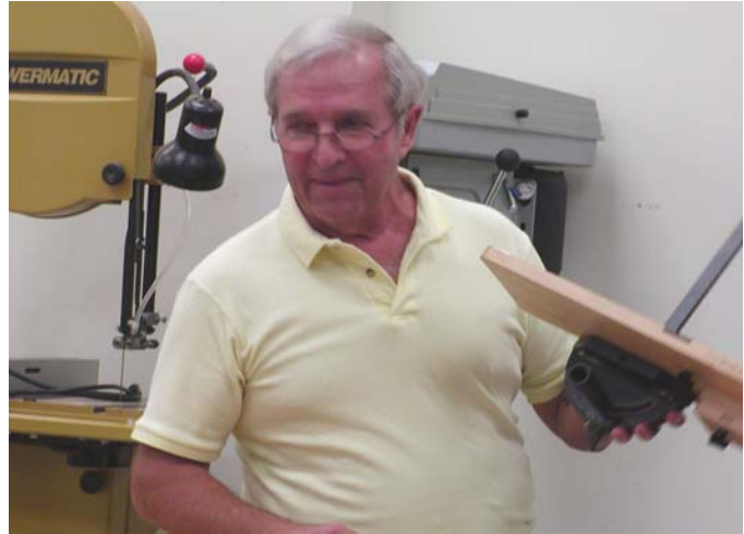
Bob Waddell demonstrated the use of this converted miter gauge to useful jig for his table saw.
