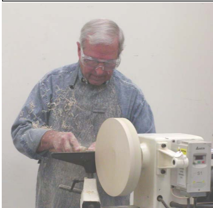
Bob Waddell (above) demonstrates his skills in turning the seat for a three-legged milling stool. Myron Curtis (below) shows how the legs are turned for the same stool.
