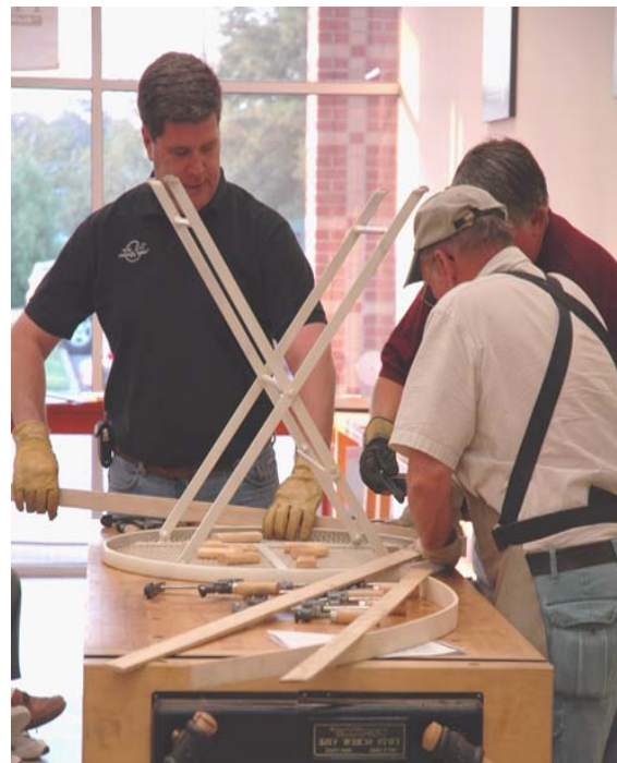
Above, Tom Smith and Bob Fred show how flexible different thicknesses of woods retain their bent capabilities after time in the steamer. To the right, a group effort is required as well as insulated gloves when bending and clamping hot, steamed wood around a shape or pattern.
