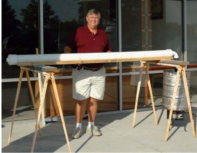
Tom Smith, above, displays the steaming tube he uses to soften wood for the wood bending demonstration. For those of you who came early found out that this tube is useful at tailgate parties as a hot dog steamer. Bob Fred, top right, demonstrates the importance of letting the wood sit for a while in the steamer. Other wise the wood will split.
