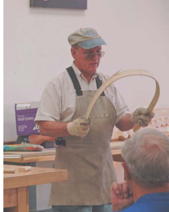
Tom Smith, above, displays the steaming tube he uses to soften wood for the wood bending demonstration. For those of you who came early found out that this tube is useful at tailgate parties as a hot dog steamer. Bob Fred, top right, demonstrates the importance of letting the wood sit for a while in the steamer. Other wise the wood will split.
