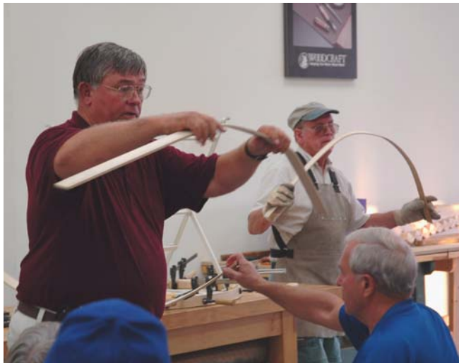
Above, Tom Smith and Bob Fred show how flexible different thicknesses of woods retain their bent capabilities after time in the steamer. To the right, a group effort is required as well as insulated gloves when bending and clamping hot, steamed wood around a shape or pattern.
